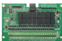
16-Relay Output Unit
