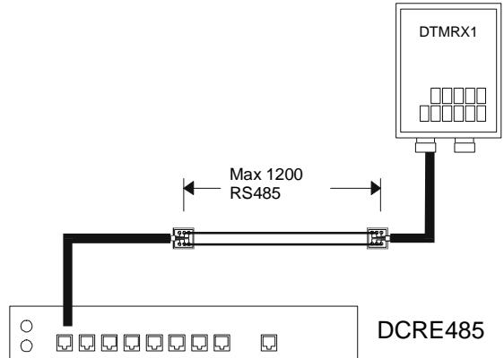
For the receivers connection to the terminal board refer to the relevant user manuals.
