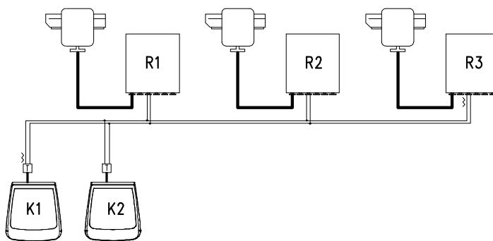
The ends (Keyboard K1- Receiver R3) should have the termination resistance inserted. Receivers R1, R2 and the keyboard K2 should not have the termination resistance inserted. The maximum length of the line, from end to end (from keyboard K1 to receiver R3), is 1200 metres.
