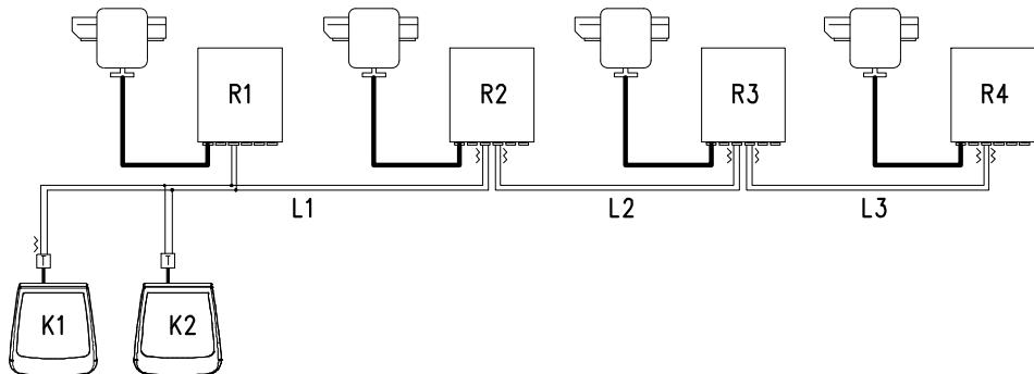
In this example, if receiver R1 is blocked (with multi-point connection in line L1) this will not cause a failure in receiver R2. R1 is not at the end of line L1, and so does not need to be terminated. If receiver R2 is blocked, as the 'generator' of the L2 line all receivers connected to it in cascade (R3 and R4) will not receive commands.
